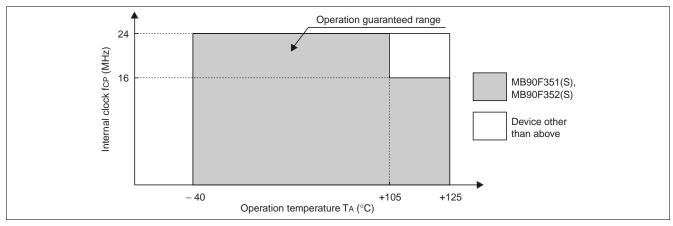
WARNING: The recommended operating conditions are required in order to ensure the normal operation of the semiconductor device. All of the device's electrical characteristics are warranted when the device is operated within these ranges.
