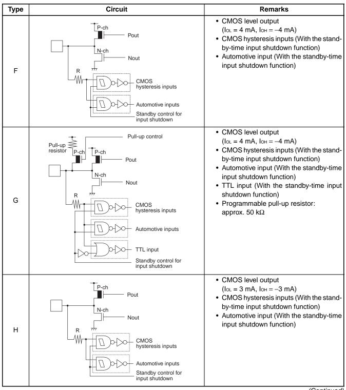
This circuit does not operate in modes where CPU operation is stopped.
