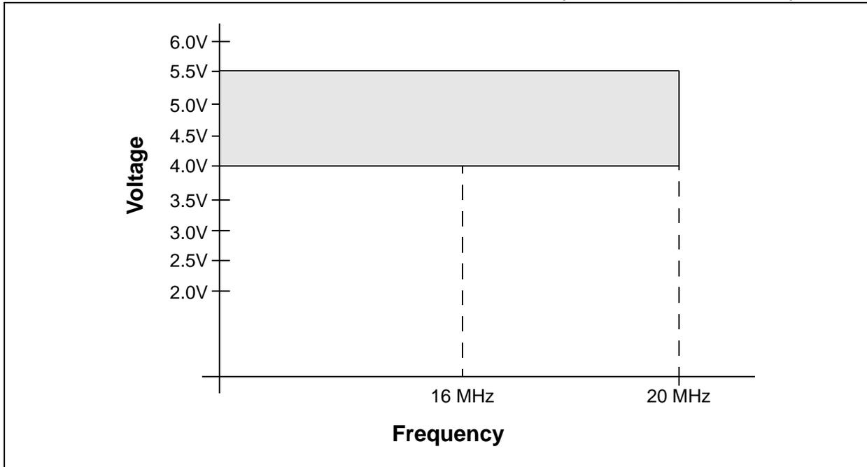
FIGURE 18-2: PIC16LF7X7 VOLTAGE-FREQUENCY GRAPH (INDUSTRIAL)
