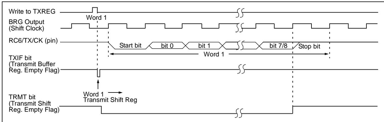
**FIGURE 11-3: ASYNCHRONOUS MASTER TRANSMISSION (BACK TO BACK)**
