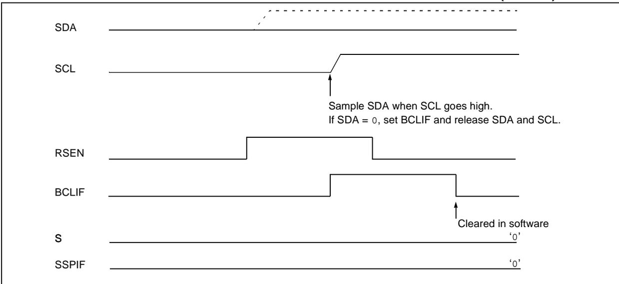
**FIGURE 10-30: BUS COLLISION DURING A REPEATED START CONDITION (CASE 2)**
