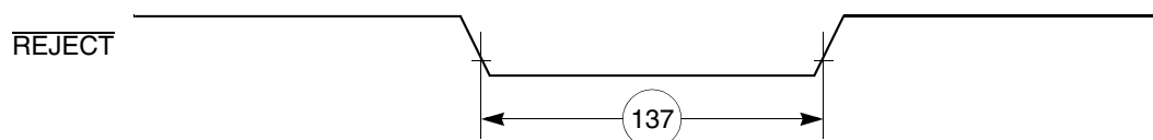
Figure 63. CAM Interface \overline{\text{REJECT}} Timing Diagram
