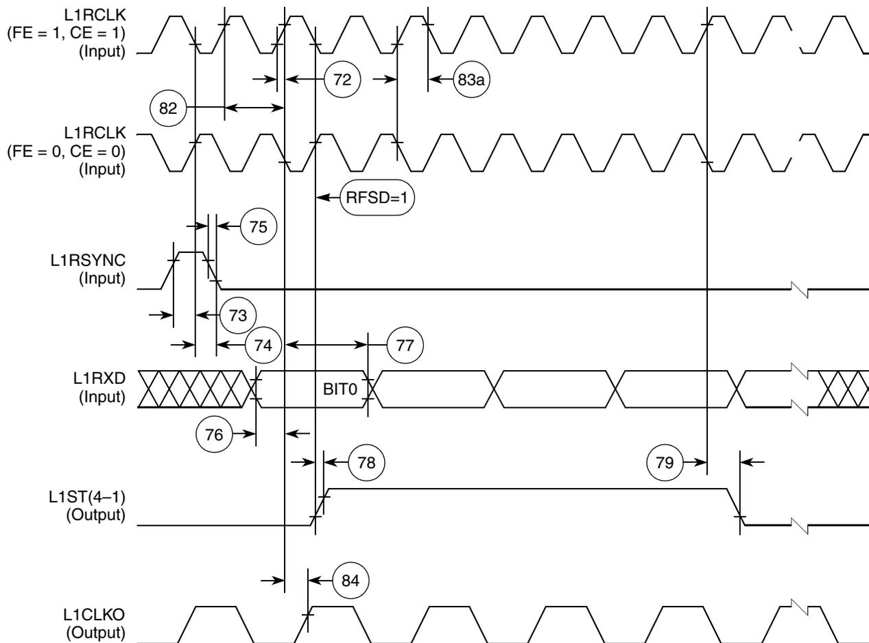
Figure 52. SI Receive Timing with Double-Speed Clocking (DSC = 1)
