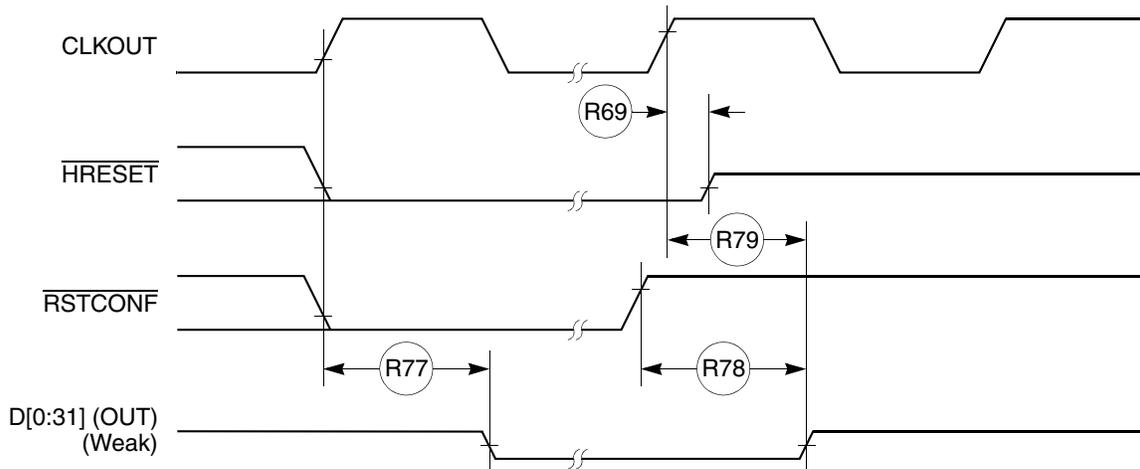
**Figure 33. Reset Timing—Data Bus Weak Drive During Configuration**
