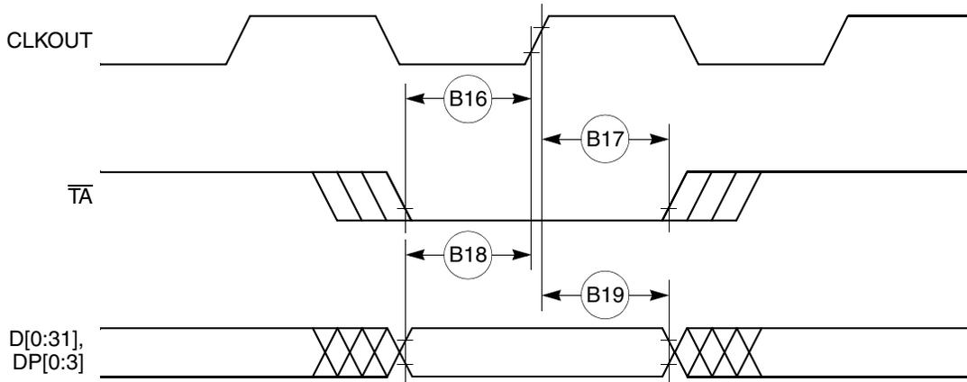
Figure 8. Input Data Timing in Normal Case
