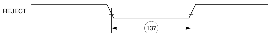
Figure 63. CAM Interface \overline{\text{REJECT}} Timing Diagram
