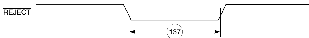
Figure 63. CAM Interface \overline{\text{REJECT}} Timing Diagram
