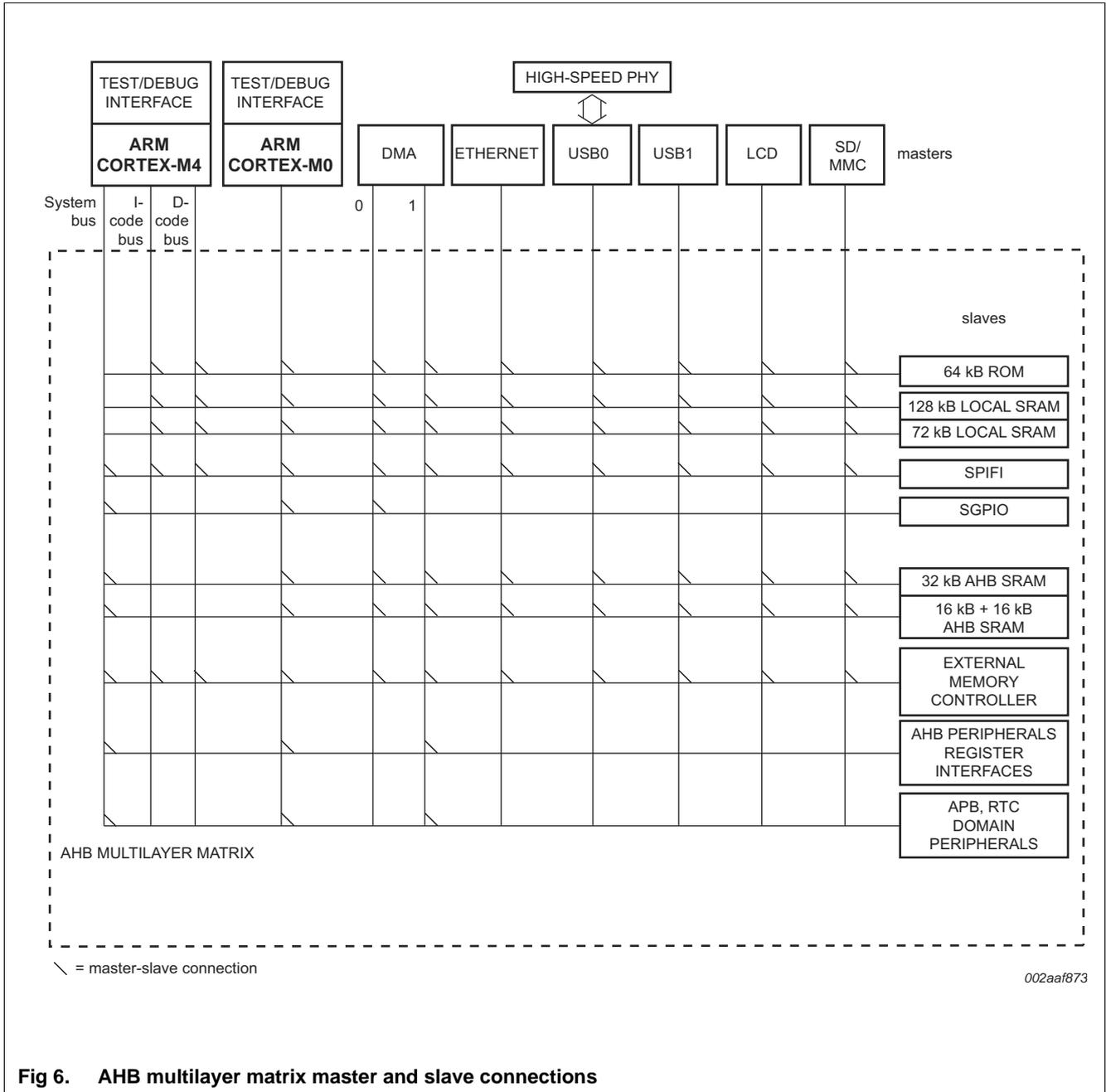
Fig 6. AHB multilayer matrix master and slave connections
