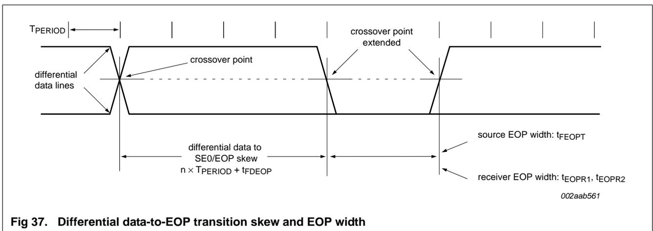
Fig 37. Differential data-to-EOP transition skew and EOP width
