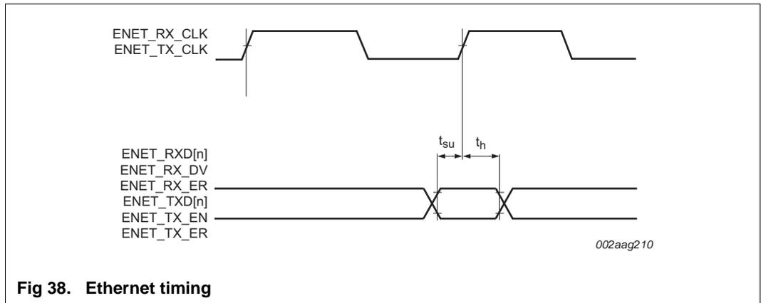
**Fig 38. Ethernet timing**
