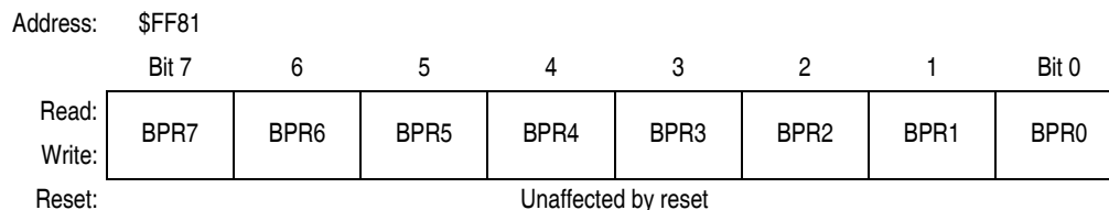
Figure 2-8. FLASH-2 Block Protect Register (FL2BPR)
