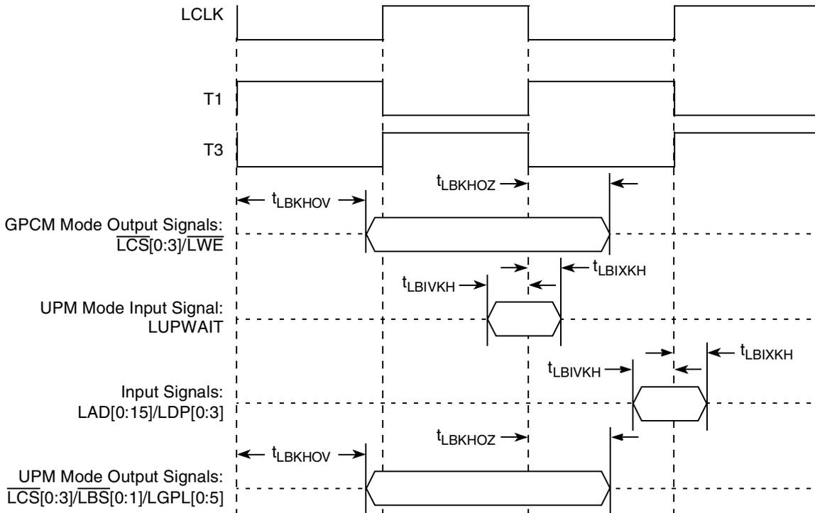
Figure 16. Local Bus Signals, GPCM/UPM Signals for LCRR[CLKDIV] = 2
