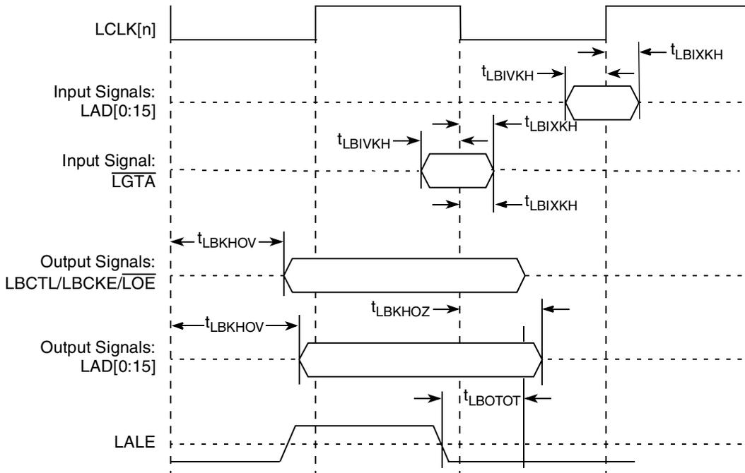
Figure 15. Local Bus Signals, Nonspecial Signals Only
