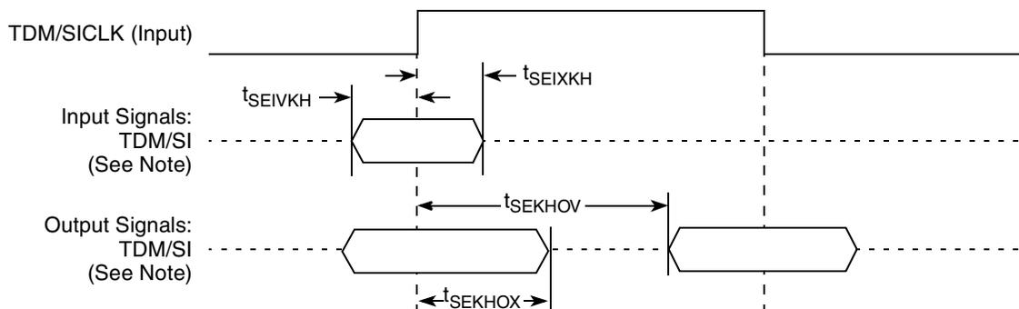
**Note:** The clock edge is selectable on TDM/SI.
