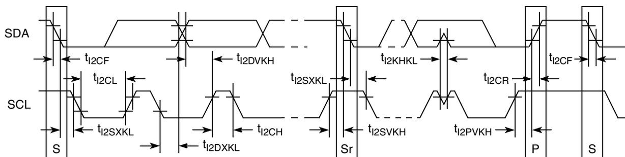
**Figure 24. I<sup>2</sup>C Bus AC Timing Diagram**
