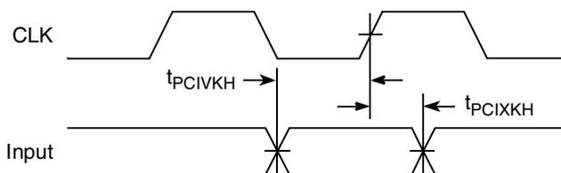
**Figure 26. PCI Input AC Timing Measurement Conditions**
