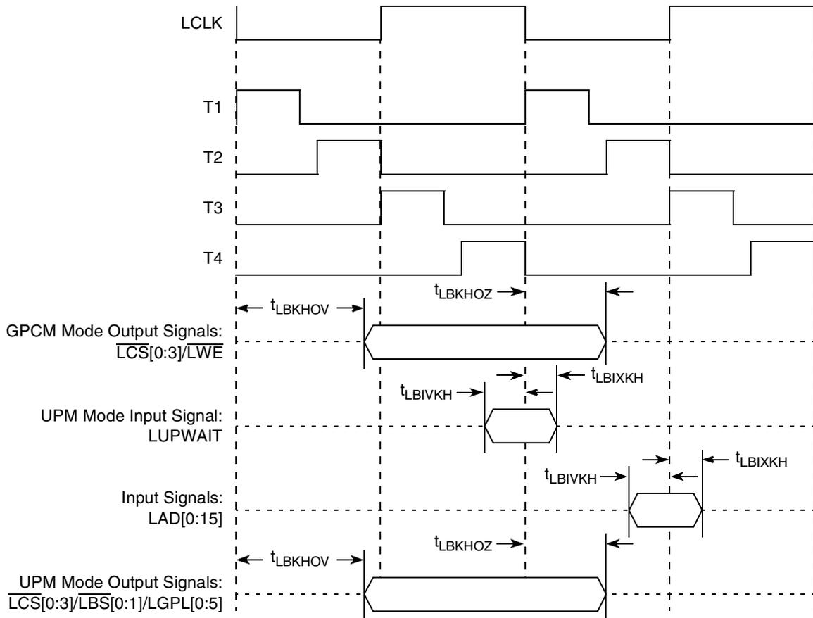
Figure 17. Local Bus Signals, GPCM/UPM Signals for LCRR[CLKDIV] = 4
