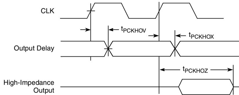
Figure 27. PCI Output AC Timing Measurement Condition
