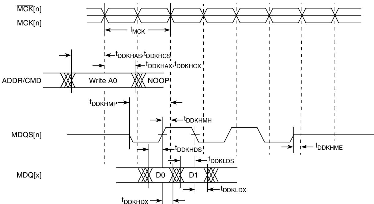
Figure 6. DDR1 and DDR2 SDRAM Output Timing Diagram
