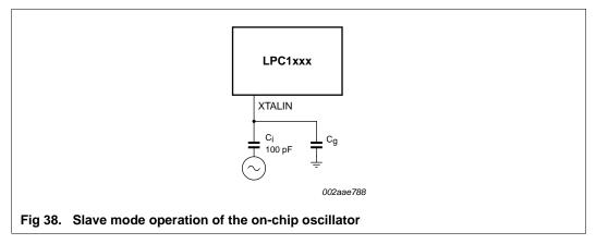
In slave mode the input clock signal should be coupled through a capacitor of 100 pF (<u>Figure 38</u>), with an amplitude between 200 mV (RMS) and 1000 mV (RMS). This corresponds to a square wave signal with a signal swing of between 280 mV and 1.4 V. The XTALOUT pin in this configuration can be left unconnected.
