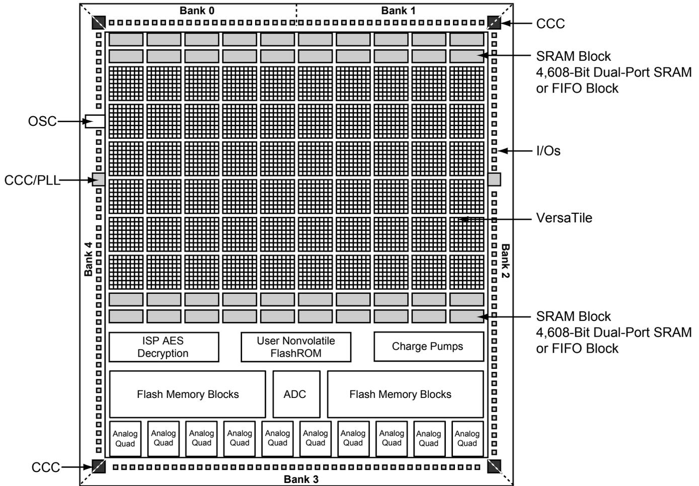
Figure 1 • Fusion Device Architecture Overview (AFS600)
