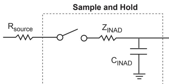
**Figure 2-88 • Simplified Sample and Hold Circuitry**
