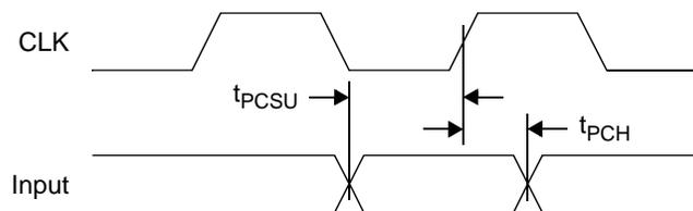
**Figure 16. PCI Input AC Timing Measurement Conditions**
