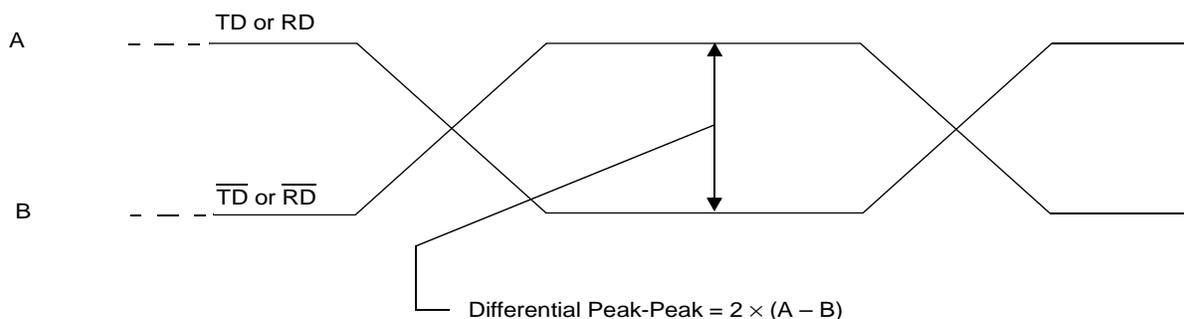
Figure 11. Differential  $V_{\text{PP}}$  of Transmitter or Receiver
