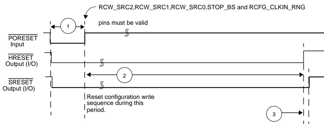
**Figure 7. Timing for a Reset Configuration Write**
