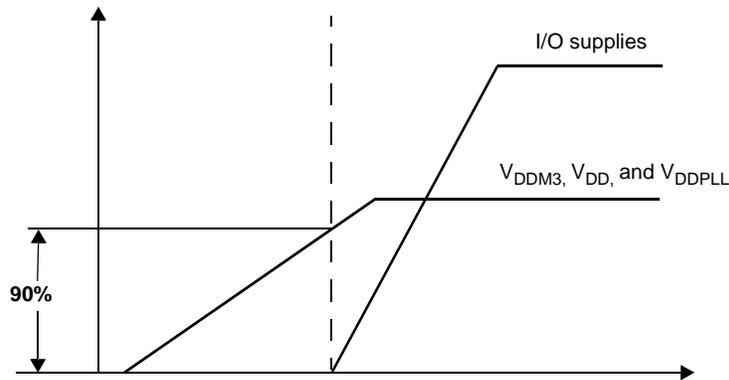
Figure 42.  $V_{DDM3}$ ,  $V_{DDM3IO}$  and  $V_{25M3}$  Power-on Sequence
