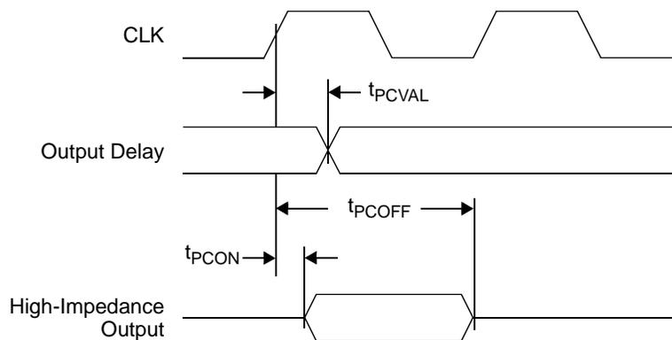
**Figure 17. PCI Output AC Timing Measurement Condition**
