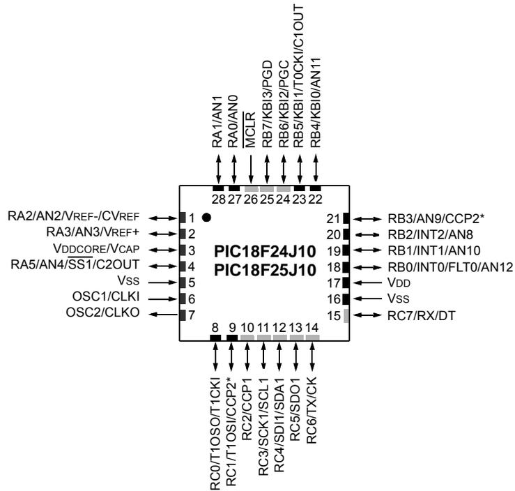
\* Pin feature is dependent on device configuration.
