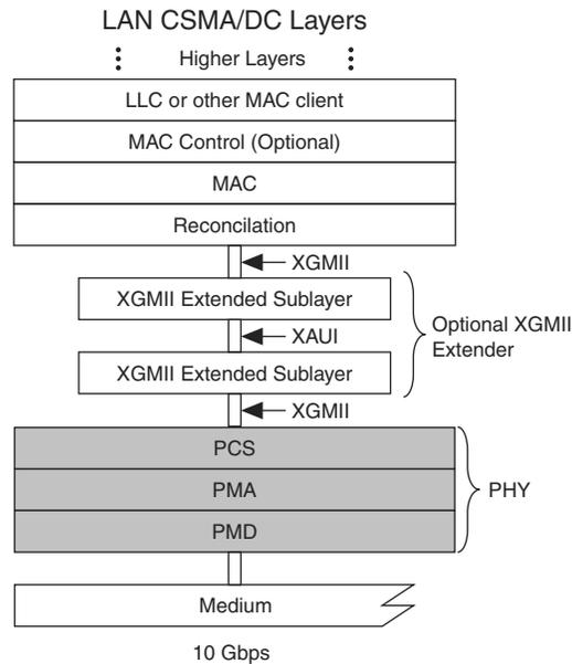
XAUI functions as a self-managed interface because code group synchronization, channel deskew, and clock domain decoupling is handled with no upper layer support requirements. This functionality is based on the PCS code groups that are used during the inter-packet gap time and idle periods.
