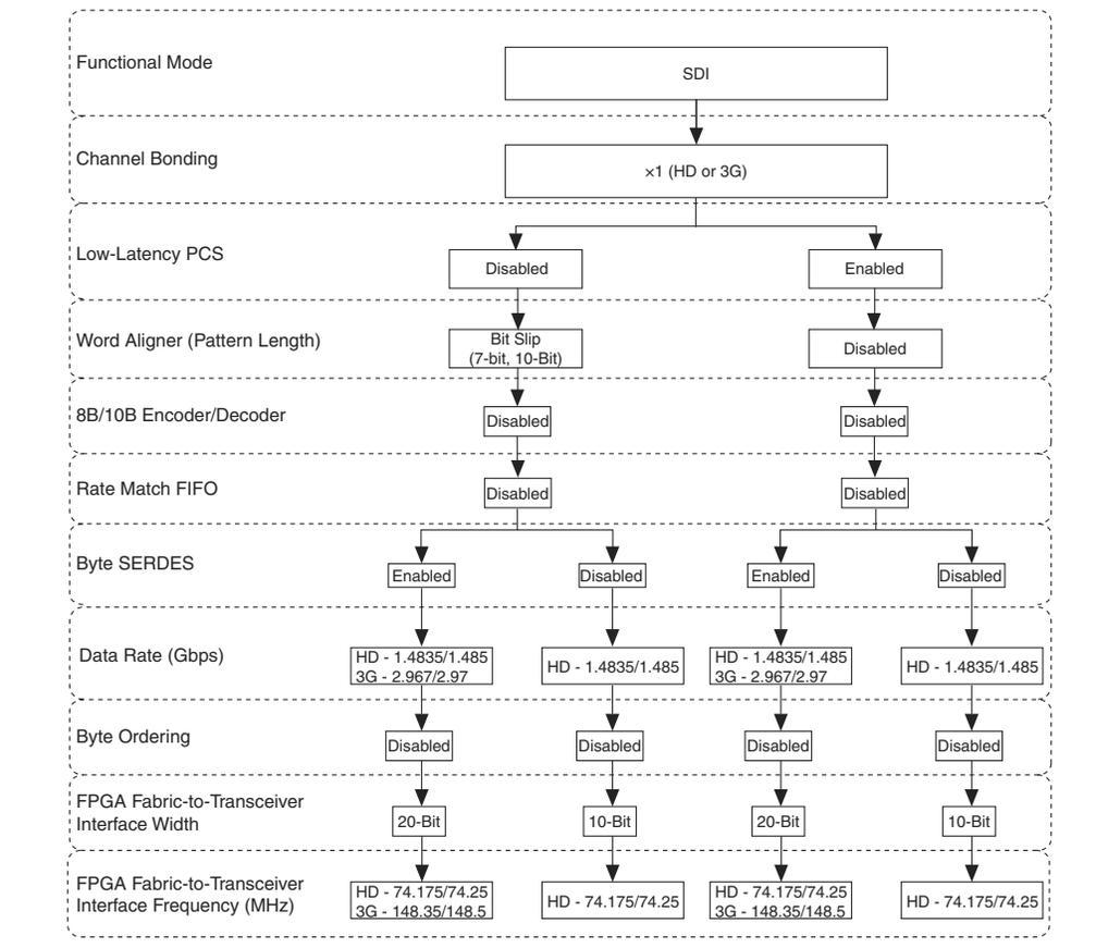
Altera recommends driving `rx_bitslip` port low in configuration where low-latency PCS is not enabled. In SDI systems, the word alignment and framing occurs after descrambling, which is implemented in the user logic. The word alignment therefore is not useful, and keeping `rx_bitslip` port low avoids the word aligner from inserting bits in the received data stream.
