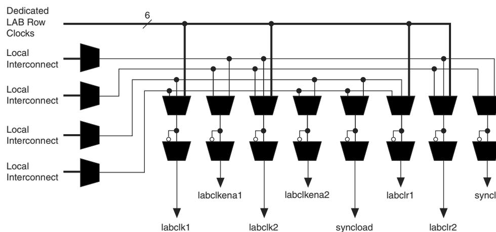
LAB-wide signals control the logic for the clear signal of the register. The LE directly supports an asynchronous clear function. Each LAB supports up to two asynchronous clear signals (`labclr1` and `labclr2`).
