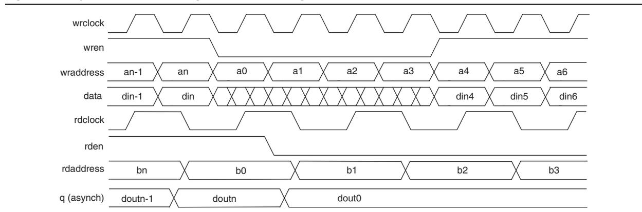
In this mode, you also have two output choices: **Old Data** mode or **Don't Care** mode. In **Old Data** mode, a read-during-write operation to different ports causes the RAM outputs to reflect the old data at that address location. In **Don't Care** mode, the same operation results in a “Don't Care” or unknown value on the RAM outputs.
