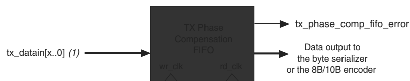
Figure 1–4. TX Phase Compensation FIFO Block Diagram
