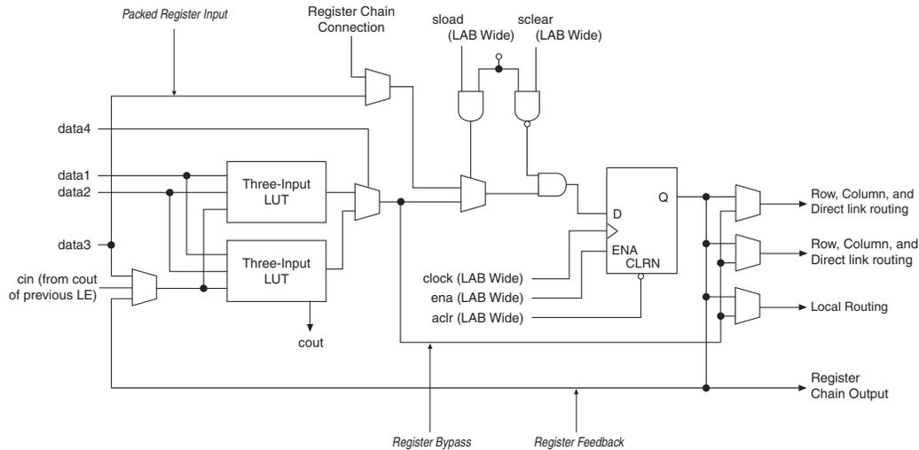
The Quartus II Compiler automatically creates carry chain logic during design processing. You can also manually create the carry chain logic during design entry. Parameterized functions, such as LPM functions, automatically take advantage of carry chains for the appropriate functions.
