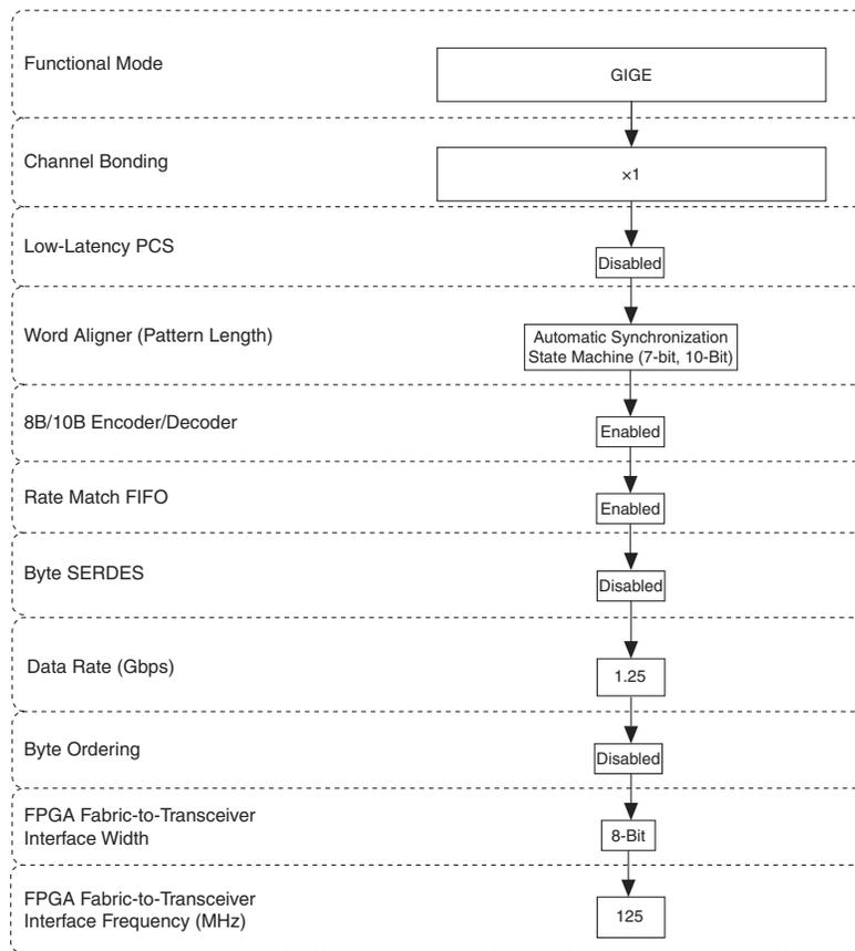
When configured in GIGE mode, three encoded comma (/K28.5/) code groups are transmitted automatically after deassertion of `tx_digitalreset` and before transmitting user data on the `tx_datain` port. This could affect the synchronization state machine behavior at the receiver.
