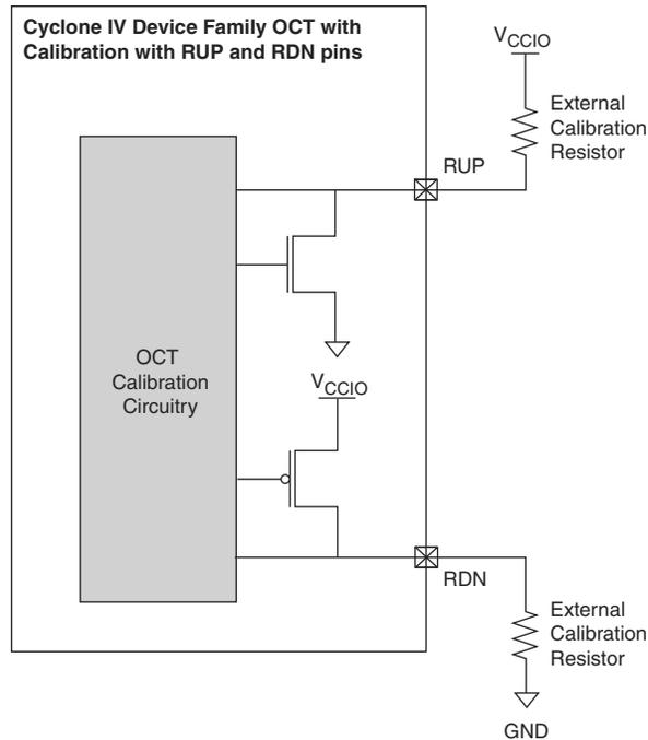
RUP and RDN pins go to a tri-state condition when calibration is completed or not running. These two pins are dual-purpose I/Os and function as regular I/Os if you do not use the calibration circuit.
