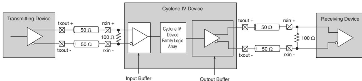
Figure 6-13 shows a point-to-point LVDS interface with Cyclone IV devices LVDS using two single-ended output buffers and external resistors.
