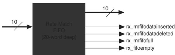
The rate match FIFO compensates for small clock frequency differences of up to  $\pm 300$  ppm (600 ppm total) between the upstream transmitter and the local receiver clocks by performing the following functions:
