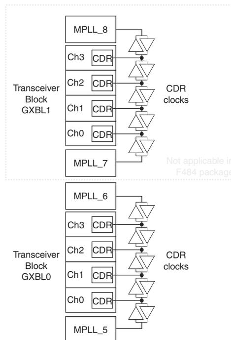
Figure 1-36 and Figure 1-37 show the independent high-speed clock and bonded low-speed clock distributions for transceivers in F324 and smaller packages, and in F484 and larger packages in bonded ( $\times 2$  and  $\times 4$ ) channel configuration.
