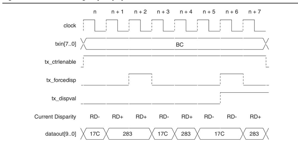
In this example, a series of K28.5 code groups are continuously sent. The stream alternates between a positive disparity K28.5 (RD+) and a negative disparity K28.5 (RD-) to maintain a neutral overall disparity. The current running disparity at time  $n + 1$  indicates that the K28.5 in time  $n + 2$  should be encoded with a negative disparity. Because tx\_forcedisp is high at time  $n + 2$ , and tx\_dispval is low, the K28.5
