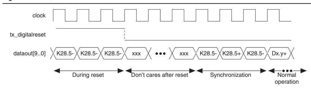
The encoder supports forcing the running disparity to either positive or negative disparity with tx\_forcedisp and tx\_dispval ports. Figure 1-8 shows an example of tx\_forcedisp and tx\_dispval port use, where data is shown in hexadecimal radix.
