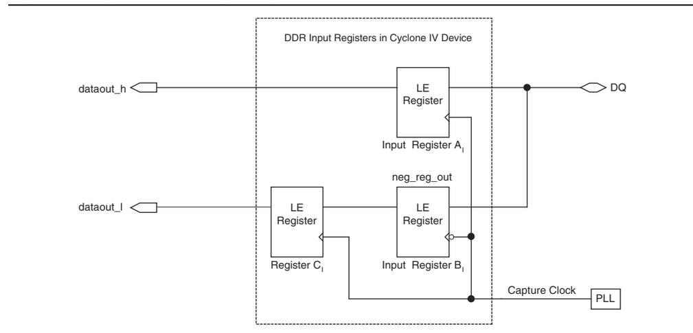
These DDR input registers are implemented in the core of devices. The DDR data is first fed to two registers, input register A<sub>1</sub> and input register B<sub>1</sub>.
