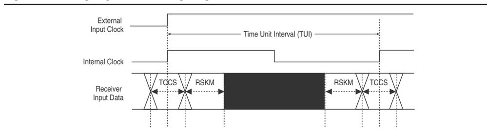
Figure 6-22 shows the Cyclone IV devices high-speed I/O timing budget.
