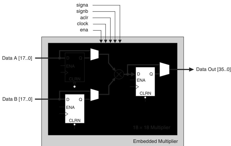
All 18-bit multiplier inputs and results are independently sent through registers. The multiplier inputs can accept signed integers, unsigned integers, or a combination of both. Also, you can dynamically change the *signa* and *signb* signals and send these signals through dedicated input registers.
