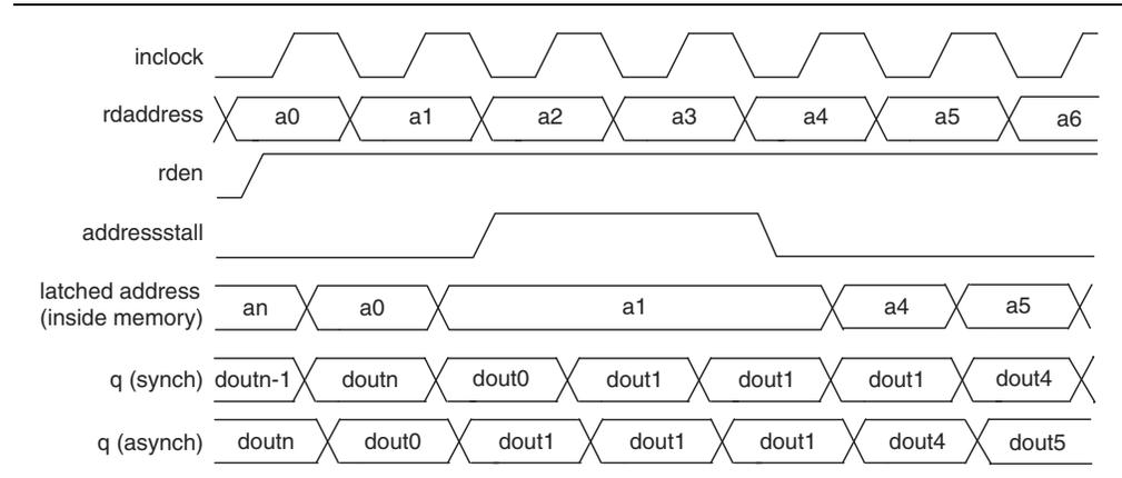
**Figure 3-4. Cyclone IV Devices Address Clock Enable During Write Cycle Waveform**
