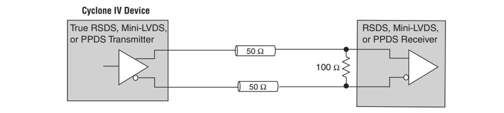
Figure 6–16 shows an RSDS, mini-LVDS, or PPDS interface with two single-ended output buffers and external resistors.
