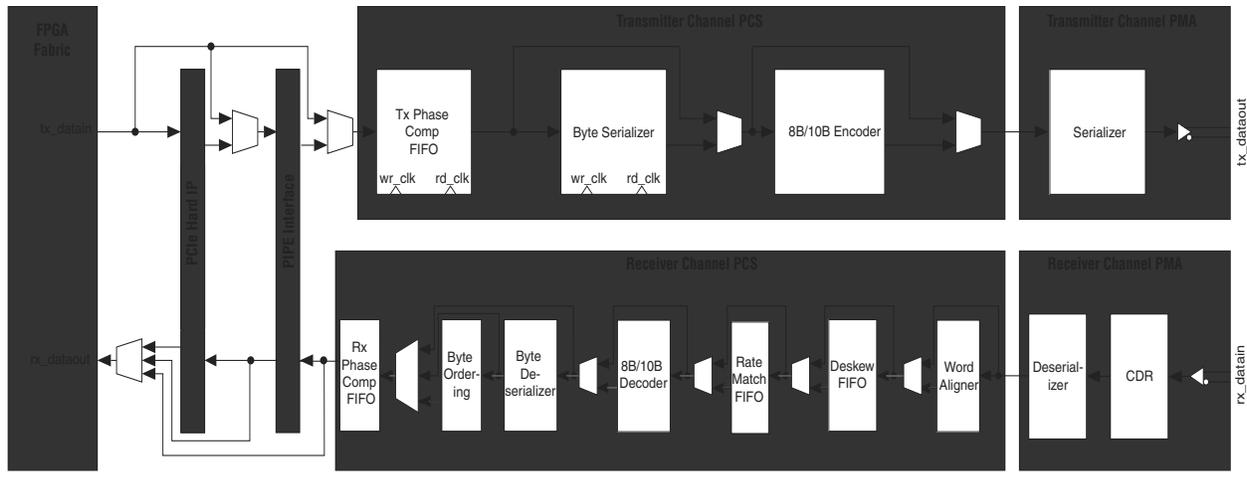
Each transceiver channel consists of a transmitter and a receiver datapath. Each datapath is further structured into the following:
