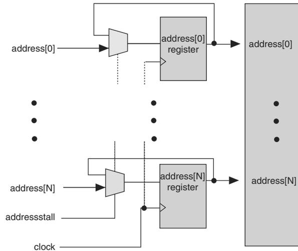
The address clock enable is typically used to improve the effectiveness of cache memory applications during a cache-miss. The default value for the address clock enable signals is low.
