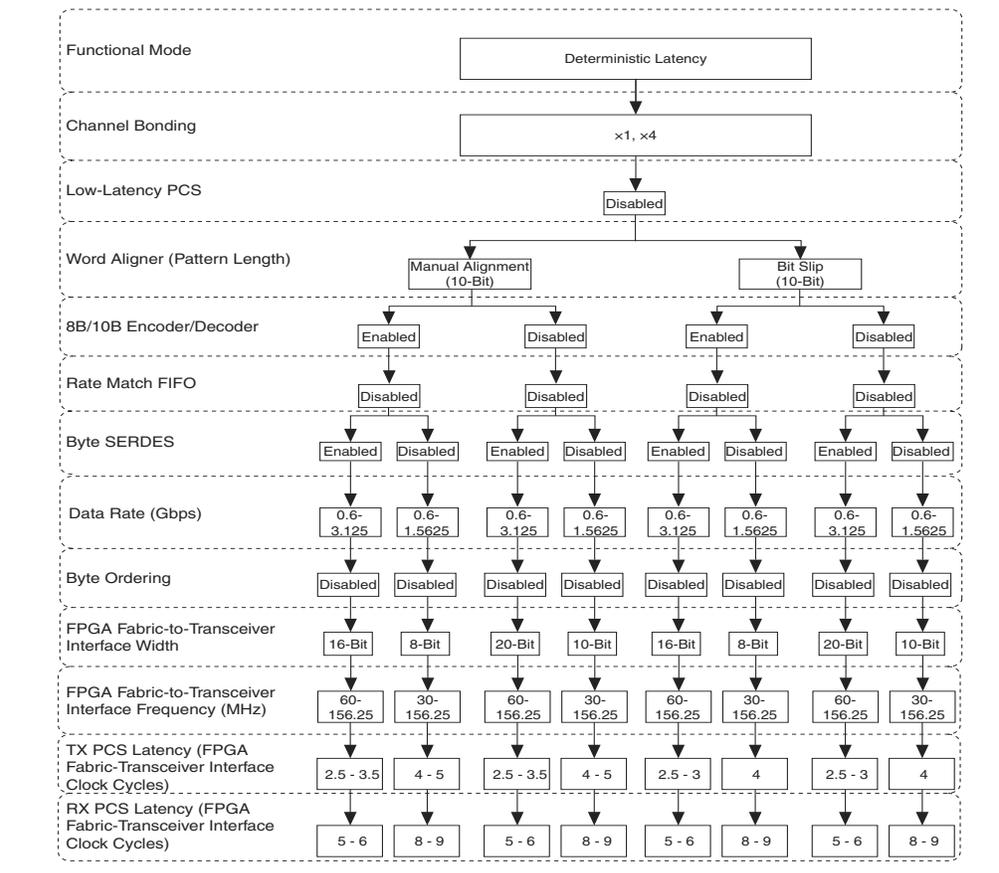
Both CPRI and OBSAI protocols define the serial interface connecting the base station component (specifically channel cards) and remote radio heads (specifically radio frequency cards) in a radio base station system with fiber optics. The protocols require the accuracy of round trip delay measurement for single-hop and multi-hop connections to be within  $\pm 16.276$  ns. The Cyclone IV GX transceivers support the following CPRI and OBSAI line rates using Deterministic Latency mode:
