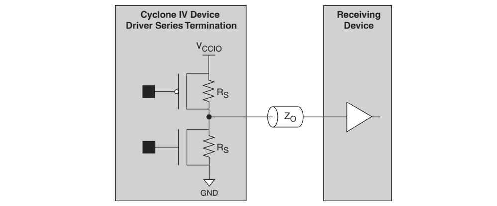
All I/O banks and I/O pins support impedance matching and series termination. Dedicated configuration pins and JTAG pins do not support impedance matching or series termination.
