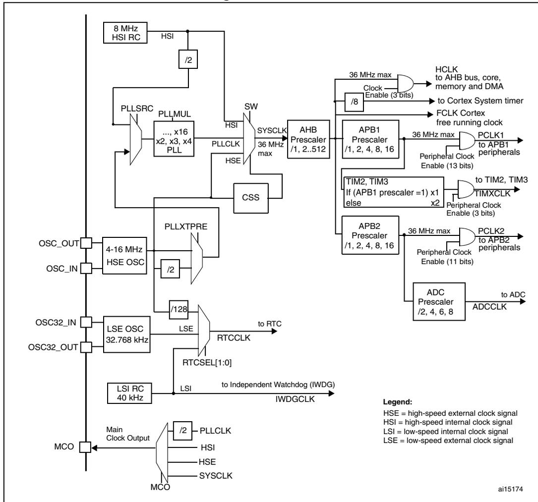
1. When the HSI is used as a PLL clock input, the maximum system clock frequency that can be achieved is 36 MHz.
