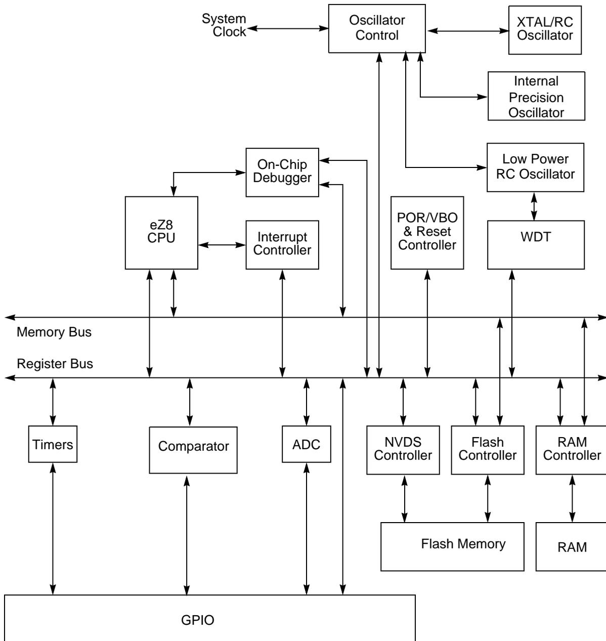
Figure 1. Z8 Encore! F0830 Series Block Diagram
