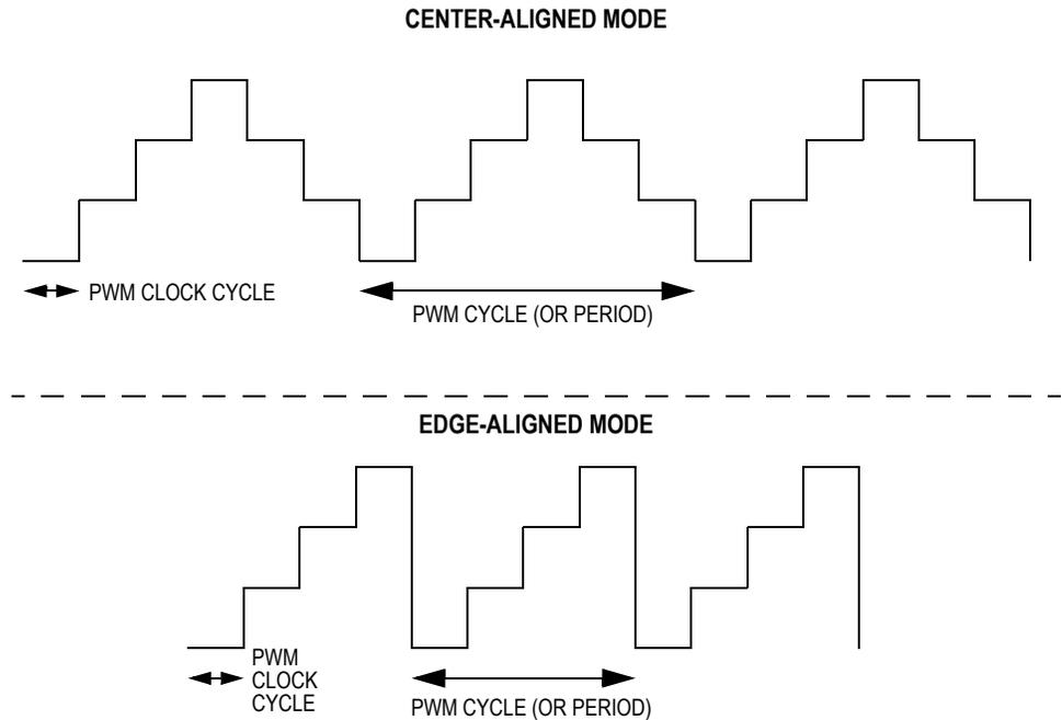
**Figure 9-43. PWM Clock Cycle and PWM Cycle Definitions**
