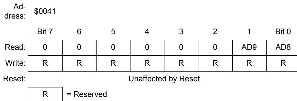
Figure 18-5. ADC Data Register High (ADRH) Right Justified Mode
