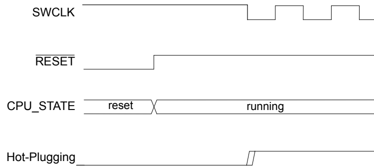
Figure 15-3. Hot-Plugging Detection Timing Diagram
