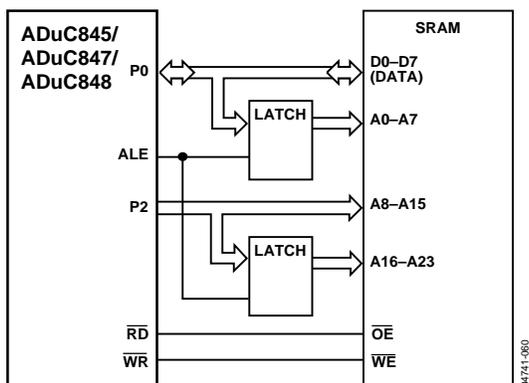
Figure 63. External Data Memory Interface (16-Mbyte Address Space)
