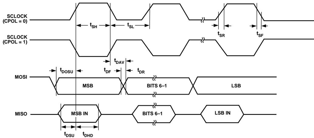
Figure 77. SPI Master Mode Timing (CPHA = 0)
