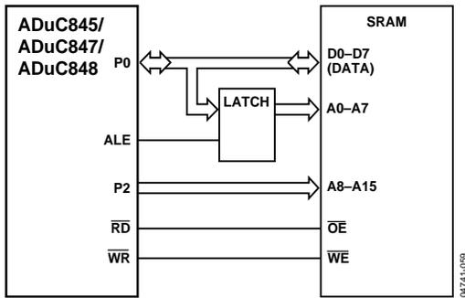
Figure 62. External Data Memory Interface (64-kbyte Address Space)
