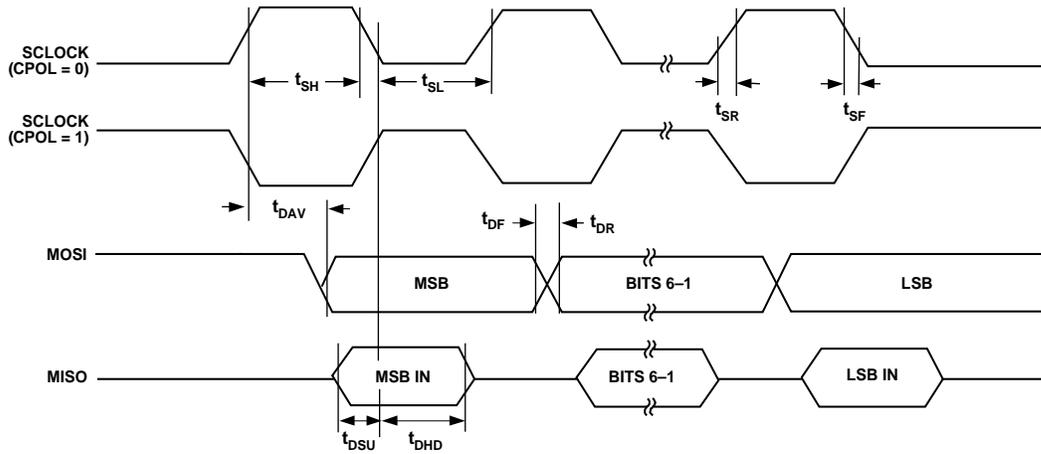
Figure 76. SPI Master Mode Timing (CHPA = 1)
