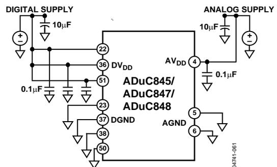
Figure 64. External Dual-Supply Connections (56-Lead LFCSP Pin Numbering)
