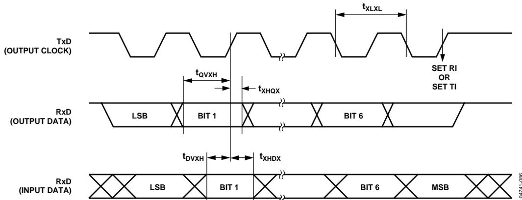
Figure 80. UART Timing in Shift Register Mode
