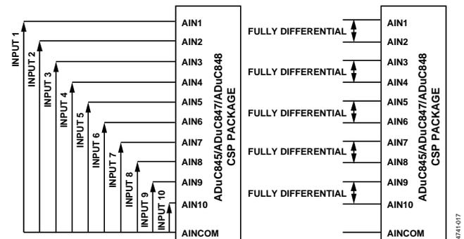
Figure 17. Unipolar and Bipolar Channel Pairs
