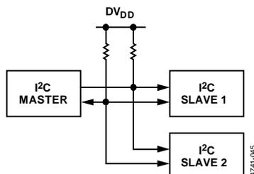
Figure 45. Typical I<sup>2</sup>C System
