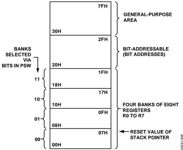
Figure 8. Lower 128 Bytes of Internal Data Memory
