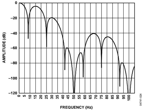
Figure 24. Chop On,  $F_{adc} = 16.6 \text{ Hz}$ ,  $SF = 52H$
