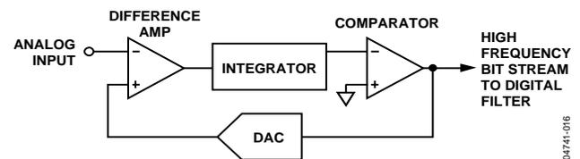
Figure 16.  $\Sigma$ - $\Delta$  Modulator Simplified Block Diagram
