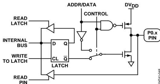
Figure 48. Port 0 Bit Latch and I/O Buffer
