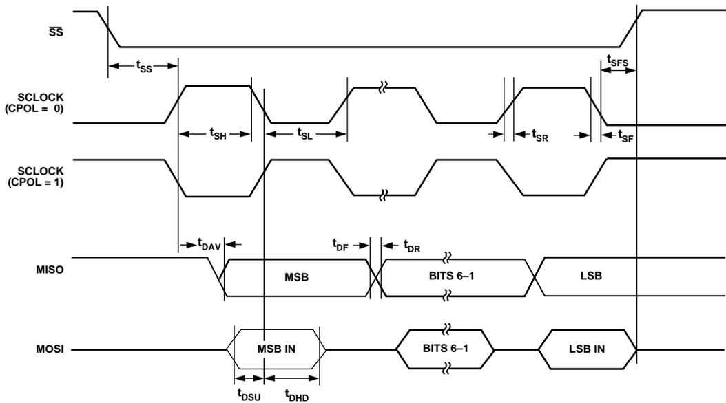
Figure 78. SPI Slave Mode Timing (CPHA = 1)
