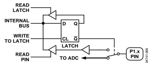
Figure 49. Port 1 Bit Latch and I/O Buffer
