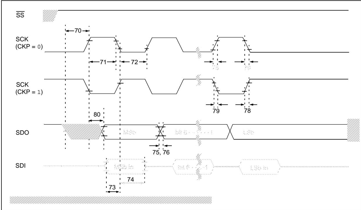
**FIGURE 27-14: EXAMPLE SPI MASTER MODE TIMING (CKE = 1)**
