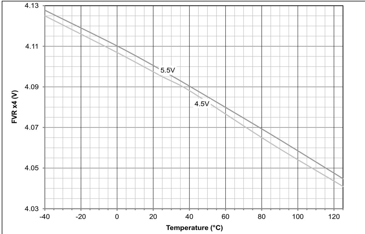
FIGURE 28-99: PIC18F2X/4XK22 TYPICAL FIXED VOLTAGE REFERENCE 4x OUTPUT
