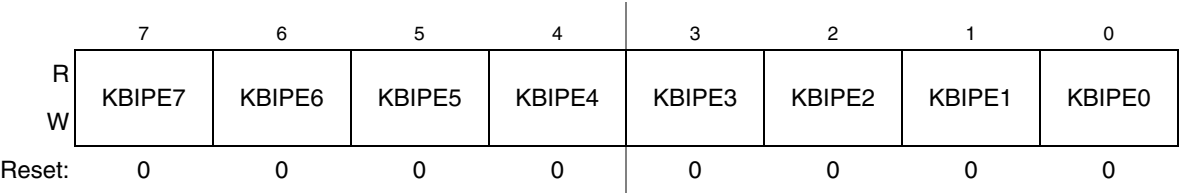
Figure 10-4. KBI Pin Enable Register
