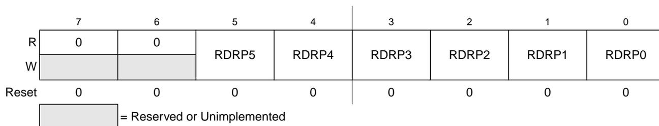
**Figure 4-26. Port P Reduced Drive Register (RDRP)**
