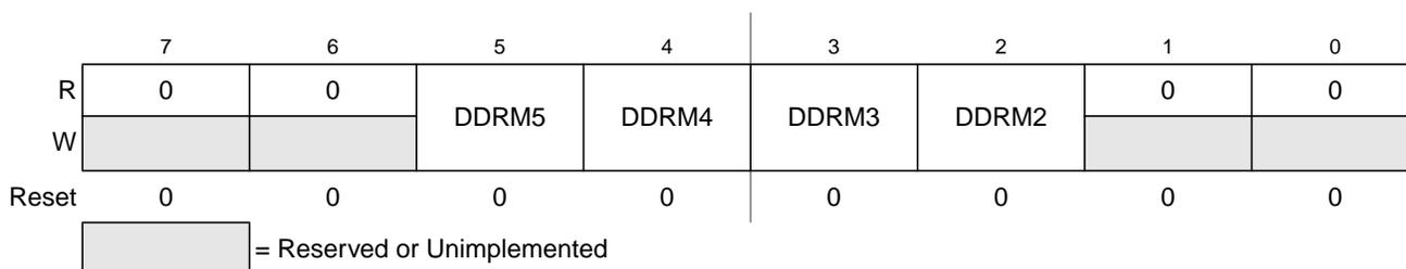
**Figure 4-18. Port M Data Direction Register (DDRM)**
