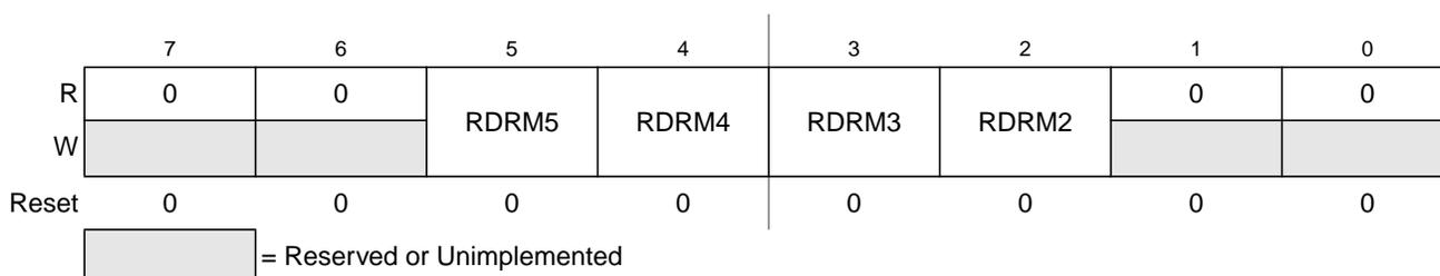
**Figure 4-19. Port M Reduced Drive Register (RDRM)**
