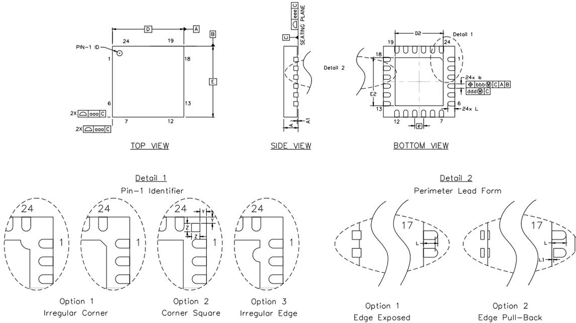
**Figure 8.1. QFN-24 Package Drawing**
