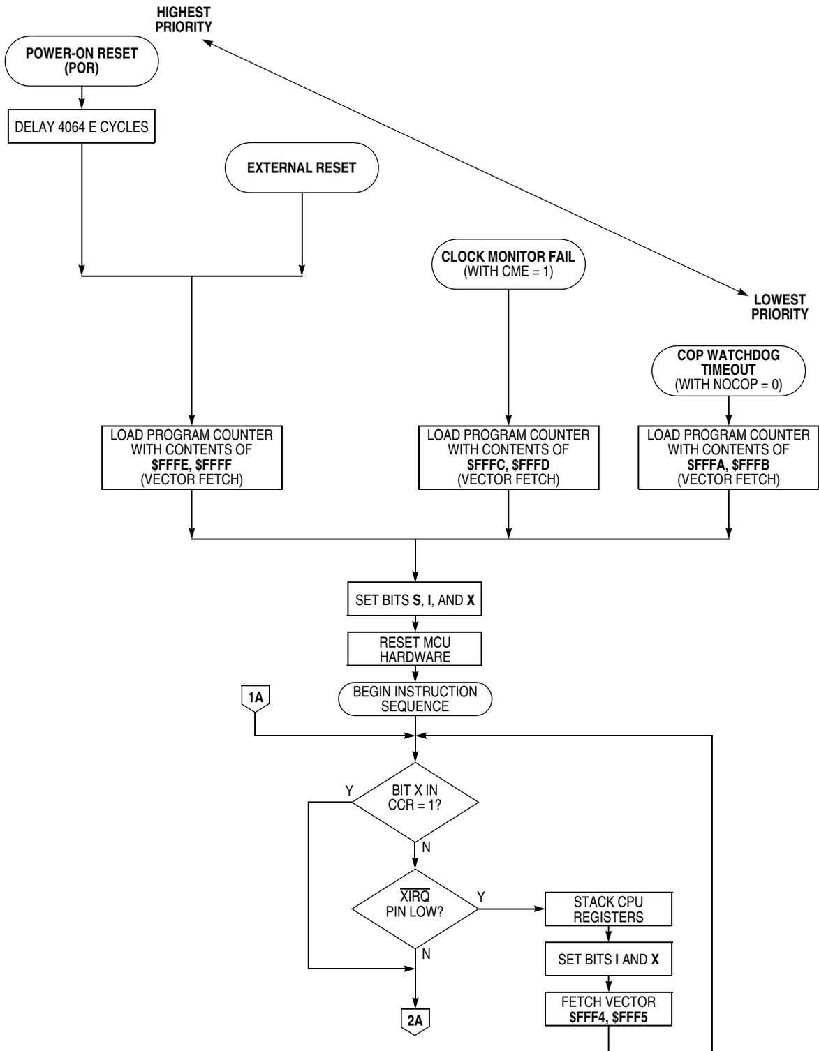
Figure 4-4. Processing Flow Out of Reset (Sheet 1 of 2)
