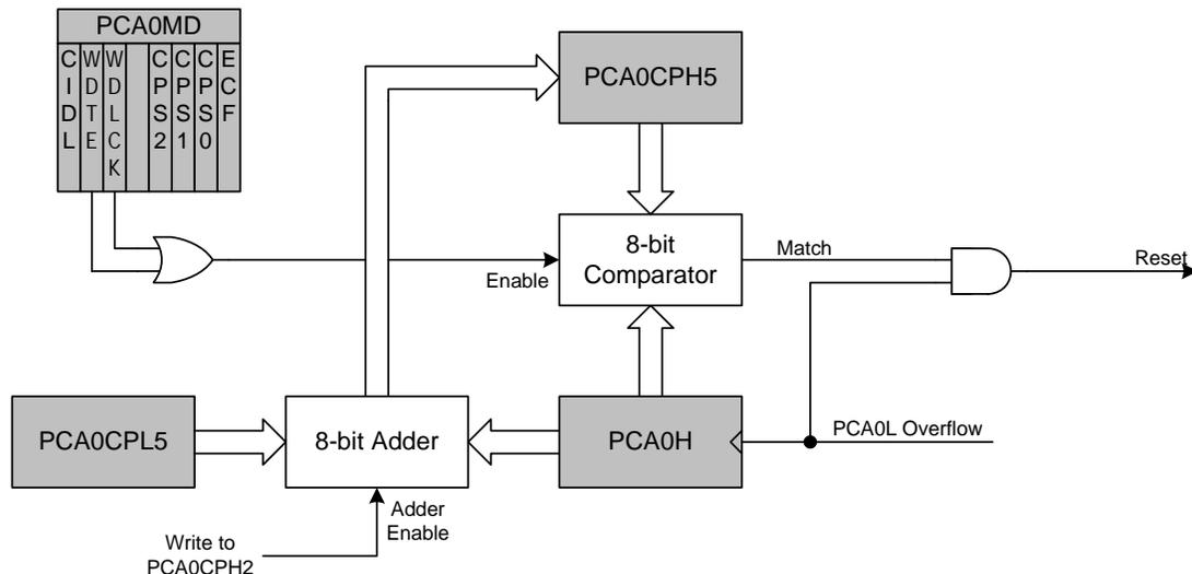
**Figure 26.11. PCA Module 2 with Watchdog Timer Enabled**
