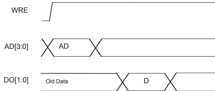
**Figure 3-14. sysCONFIG Master Serial Port Timing**
