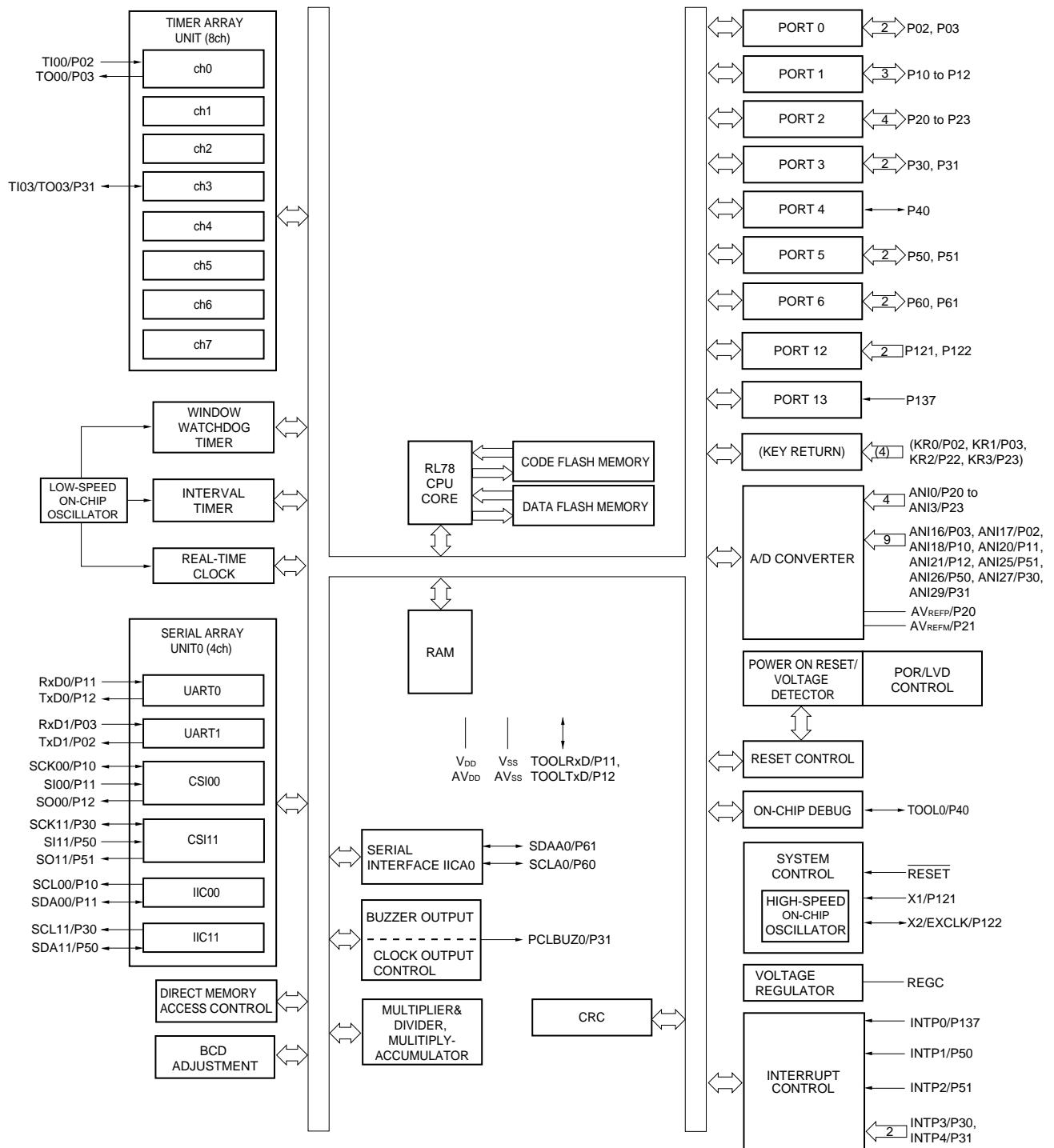
**Remark** Functions in parentheses in the above figure can be assigned via settings in the peripheral I/O redirection register (PIOR).
