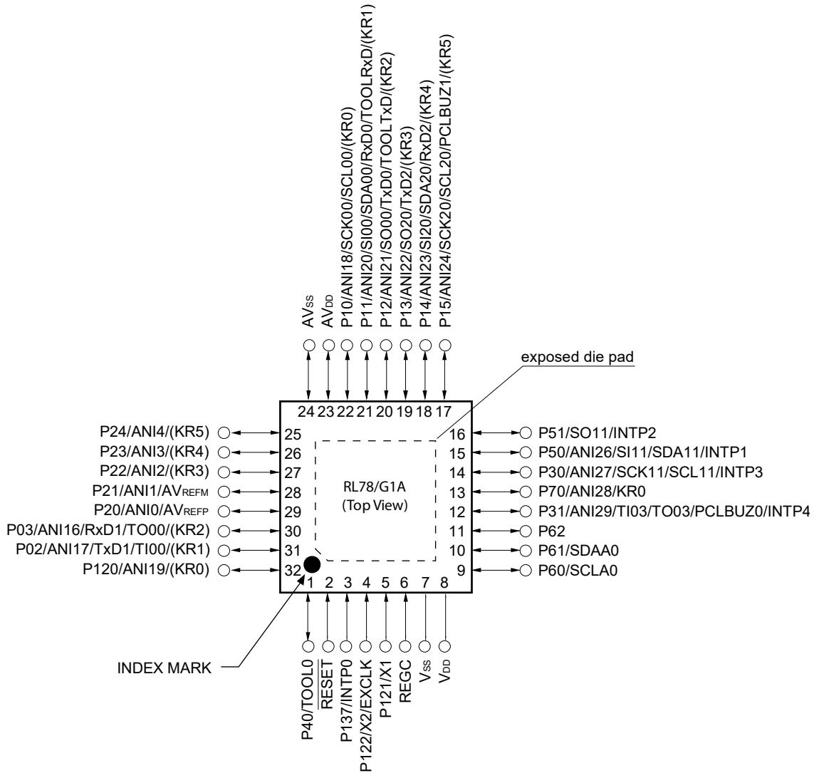
**Caution Connect the REGC pin to V<sub>ss</sub> via a capacitor (0.47 to 1 µF).**
